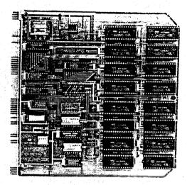
The Newburn NE889 battery-backed Static ram-disk board is an 80-Bus compatible board for use as a high-speed virtual disk ("M" drive") in all 80-Bus systems. The board is compatible with all versions of CP/M that support one or more "M" drives via I/O ports.
