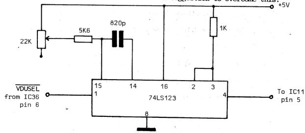
Pin 5 of IC11 should be bent out from the socket and the connections made with an insulated "soldercon" socket. Increase the potentiometer value until the flash just disappears.
