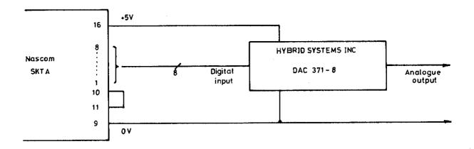
No program was written, because using the T4 Output command port A could be set up for mode 0 and no interrupt, and data written to the DAC. The long term aim is to attempt to write a Music Program, directly synthesizing music waveforms or using the analogue signal to control a voltage controlled oscillator.
